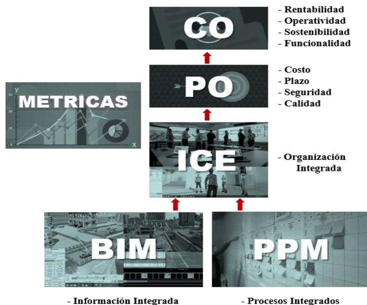
Figura 3: Estructura Virtual Design Construction (VDC).
